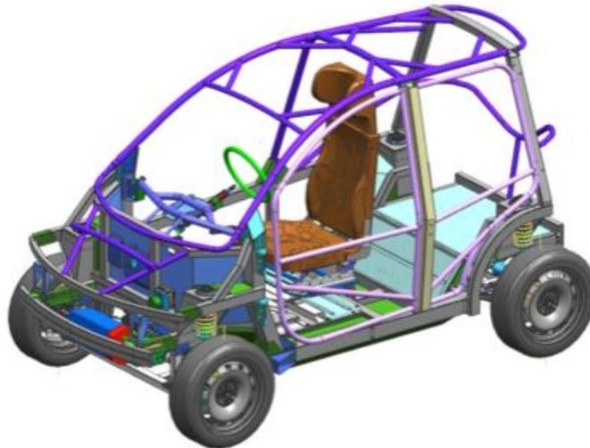
Fig. 4. The implemented tubular frame with the addition of parts made by sheet metal forming conceived for low and medium-low production volumes.
