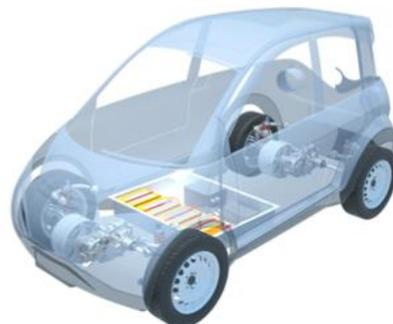
Fig. 8. Picture of the first MOB vehicle and a transparency showing the position of motors and battery pack.
