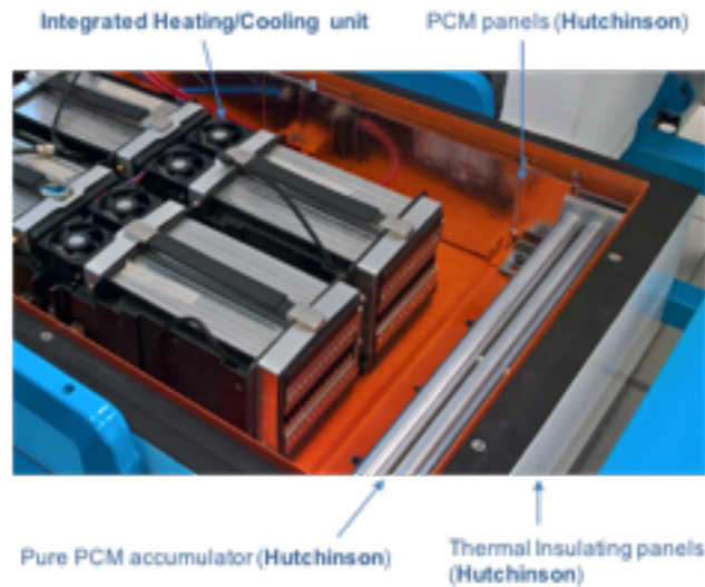
Figure 6: View of the battery pack enclosure.
